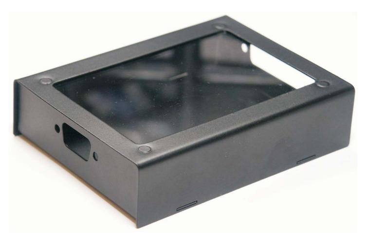
The durable steel enclosure consists of two U-shaped pieces, and requires no connecting hardware. The PCB is mounted inside the enclosure using connector screws, and has a cutout in the top side, which is covered by a transparent acrylic screen. This setup allows for easy visual access to the status LEDs.
