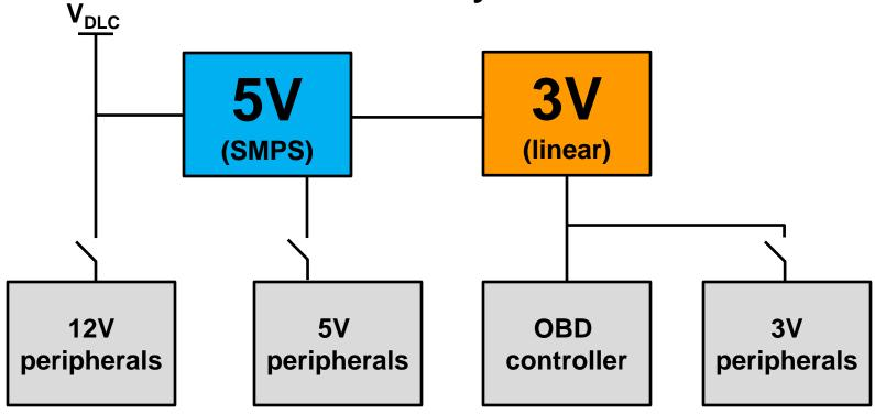
Good balance of cost, part count. Can use a low- $V_{MAX}$  regulator for 3V, low ripple on 3V rail.
