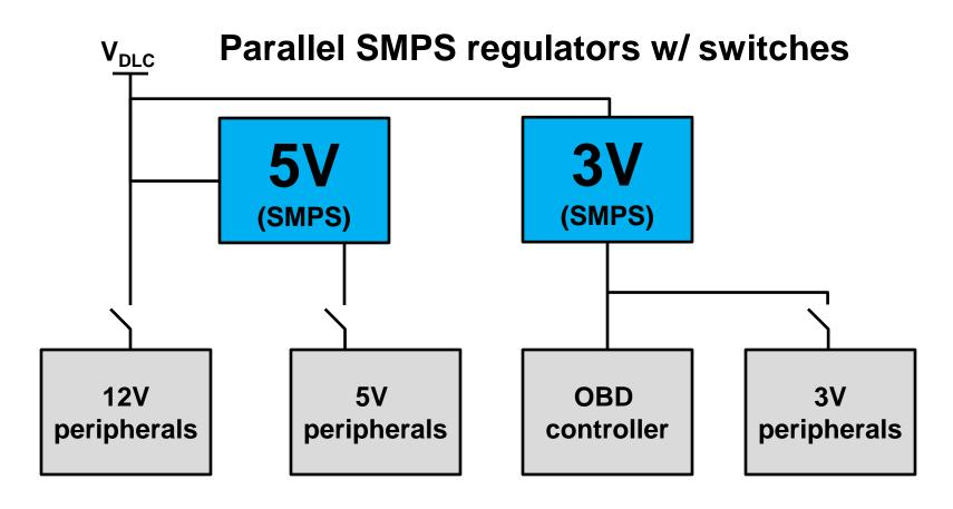
Expensive, but appropriate for applications that require high current capability on the 3V power rail.
