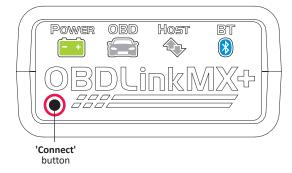
The **'BT'** LED will switch to a *fast* blink.
