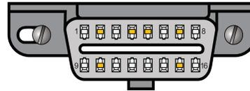
The 16-pin D-shaped diagnostic link connector (DLC) should be located in the passenger or driver's compartment in the area bounded by the driver's end of the instrument panel to 300 mm (~1 ft) beyond the vehicle centerline, attached to the instrument panel and easy to access from the driver's seat. The preferred location is between the steering column and the vehicle centerline.
