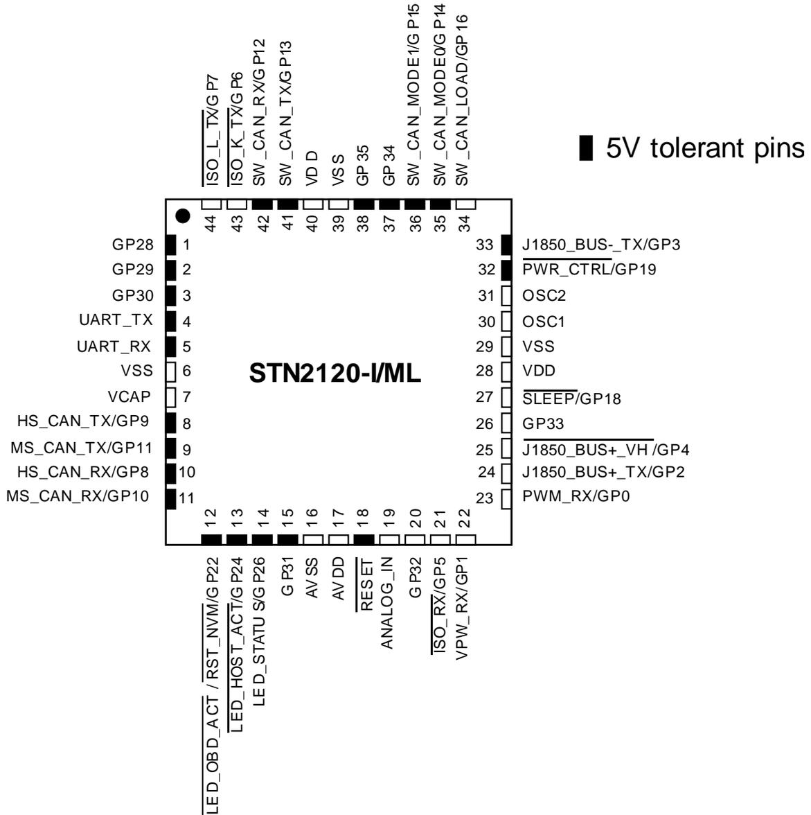
**Note** 1. The metal plane at the bottom of the device is not connected to any pins and is recommended to be connected to VSS externally.
