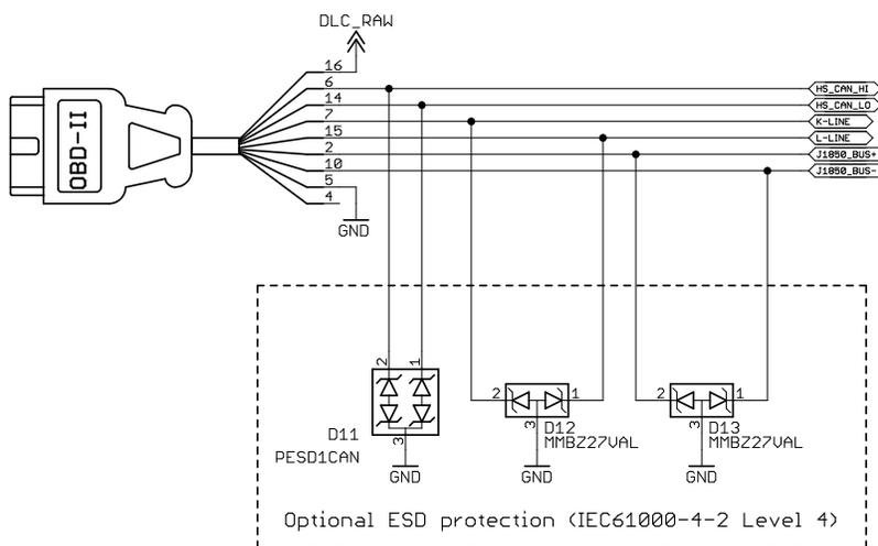
Figure 10 - STN2120 OBD Port Connector and ESD Protection
