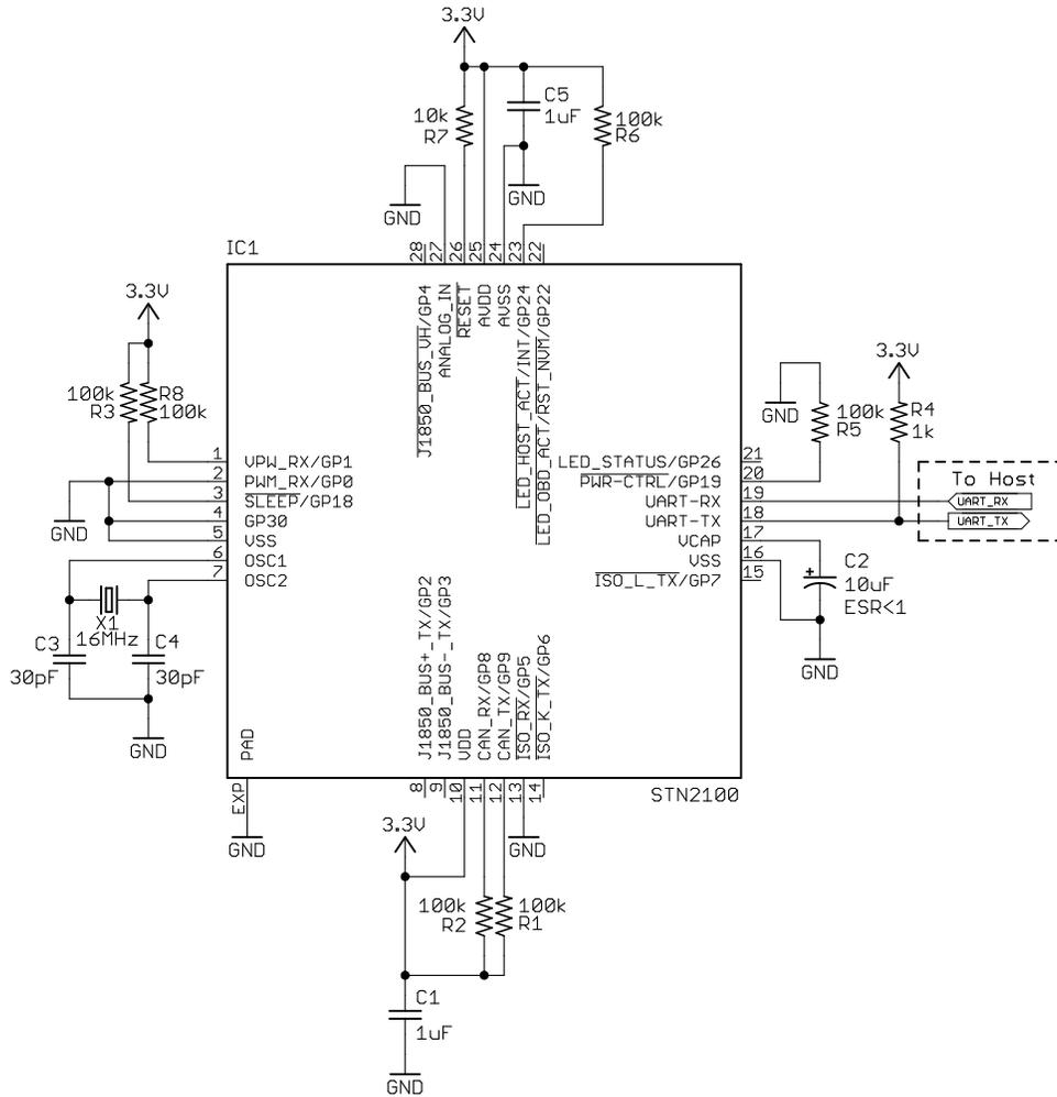
Figure 4 shows the recommended minimum of components necessary to get the STN2120 to operate reliably, while minimizing power consumption.
