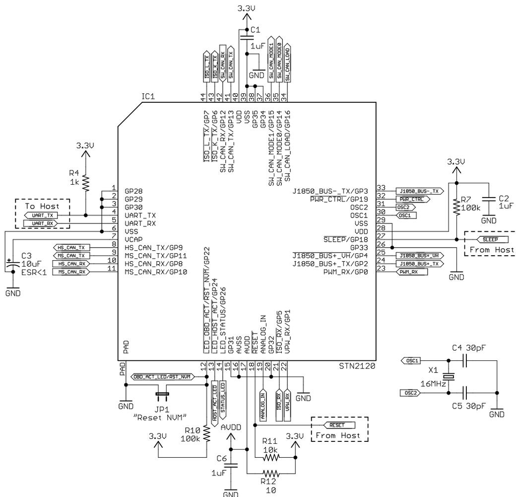
**Note 1** - Be sure to pull up RST\_NVM pin to Vdd or 5V via a 100 kΩ resistor, whether an LED is connected or not. Failure to do so may result in mysterious and unpredictable device resets.
