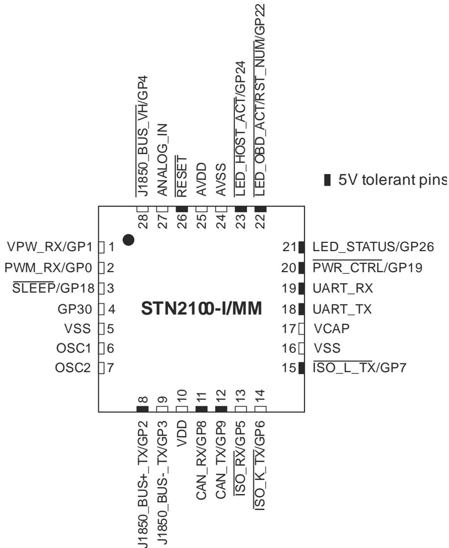
**Note** 1. The metal plane at the bottom of the device is not connected to any pins and is recommended to be connected to VSS externally.
