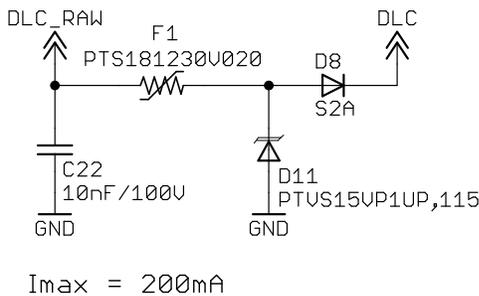
**PTC/TVS-based OVP** (Figure 11) is the simpler of the two designs, with a lower part count. In addition, this circuit may allow the load to remain powered during an overvoltage event, which may be an advantage in some situations. However, it tends to be bulkier and more expensive, especially for voltages above 60V (e.g., load dump on 24V systems) and higher operating currents.
