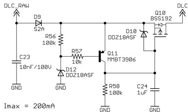
**Transistor-based OVP** (Figure 12) has a higher part count but can be physically smaller and less expensive than the PTC/TVS design.
