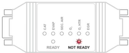
Normal connection time is between 1 and 25 seconds. If the vehicle does not reply to requests on any of the five protocols, the "Not Ready" LED will **quickly flash** five times, to indicate that it was not able to connect, and after a 20 second pause, the cycle will repeat. If connection is not established within about 60 seconds, refer to section 6 ("Troubleshooting").
