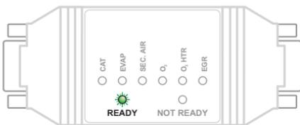
Test results will be retained for five minutes after the ignition is turned off, after which the device will enter the power-save mode, indicated by the **slowly flashing** "Ready" LED. The Ready-or-Not will periodically wake up, and attempt to reconnect.
