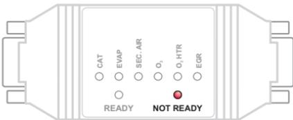
Once the connection is established, the tool will request diagnostic information from the vehicle, and display the results on the monitor status LEDs.
